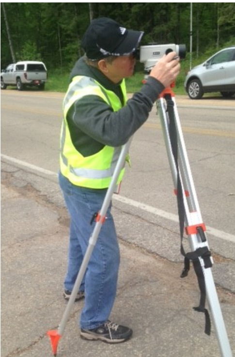
Miles Winkler, left, DNR water management engineer, lines up surveying equipment to reset water level measurements on the new culvert on Highway Y by the boat launch site. Scott Koehnke, right, DNR water management specialist, marks the elevation on the culvert. The culvert has been the official lake level bench mark, which had to be reset after the culvert was replaced last year. Official levels in feet above sea level are: marked bolt: 800.44; high water: 799.88; normal: 799.58; low: 799.28.
